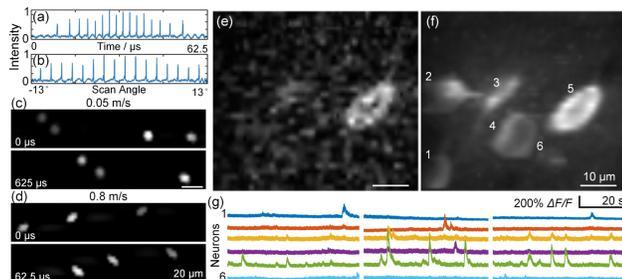
**Fig. 2.** (a), (b) Time resolved signal of a  $10 \mu\text{m}$  fluorescent bead scanned at 256 kHz line rate. (c), (d) 16 kHz imaging of flowing fluorescent beads at different speeds. Image shearing is observed at higher flow speed due to bead motion and bidirectional scanning. (e)–(g) *In vivo*  $\text{Ca}^{2+}$  imaging at 16 kHz: (e) single frame; (f) average frame of six active neurons; (g) corresponding  $\text{Ca}^{2+}$  traces over three 1 min recordings.
