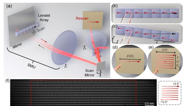
**Fig. 1.** (a) Schematic of SMU with a single-axis scanner. (b), (d) 1D scanning. (c), (e) 2D scanning. (f) 2D scanning with experimentally measured foci ( $\Theta_0 = 25^\circ$ ,  $N = 16$ ).
