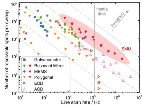
**Fig. 3.** Comparison of commercially available optical scanners without and with SMU add-on. Solid markers, inertial scanners. Empty markers, inertia-free scanners. Red solid markers, corresponding scanners with SMU add-on for  $N \in [1, 32]$ . Data points for SMU based on Cambridge Tech. CRS 8 kHz, PHCAB, and Hamamatsu Corp. S13989-01H.
